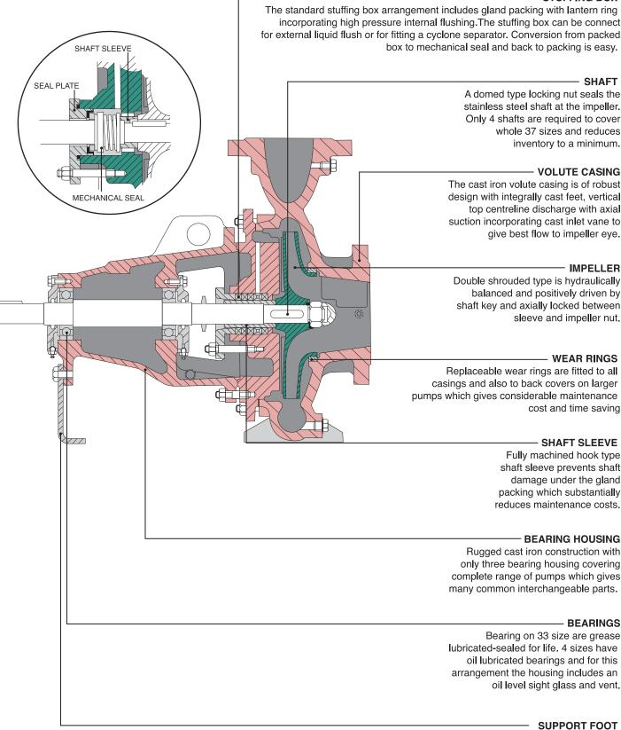
A removable support foot is fitted at the drive end for greater rigidity and ease of maintenance.
